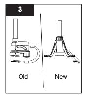
For older style Lamp Connector follow steps 4 and 5. For new Lamp Connector follow steps 6 and 7.
