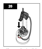
Align connection pins with the lamp connector by rotating the ring clamp.
