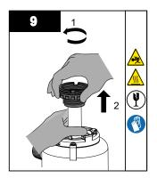
Unscrew the sleeve bolt and carefully remove it from the top of the chamber.
