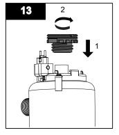
Place new (grey) sleeve bolt onto the quartz sleeve, carefully push down and hand tighten onto chamber.
