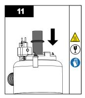
Place O-ring on the sleeve as shown. Insert the sleeve into the chamber as shown in step 12.
